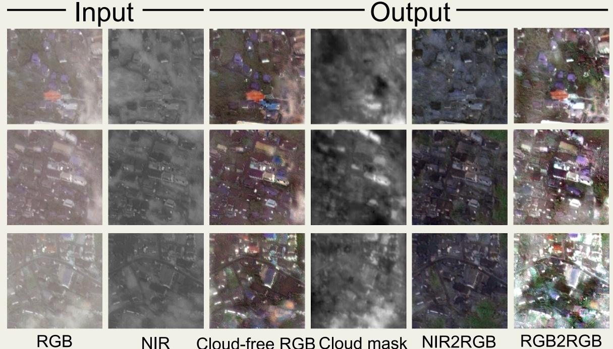
**NIR2RGB**: Color information is partially missing **RGB2RGB**: The clouds are partially removed, there are crucial errors in some results **McGANs**: The overall filmy cloud is removed
